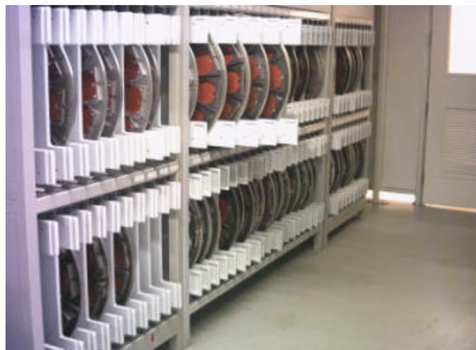
**Figure 2** The Eaton NV10 Disk Storage – Horizontal Laminar Flow Cabinet to protect the disks and to keep them clean
