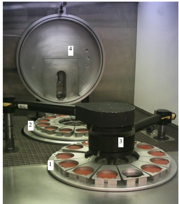
**Figure 1** The Eaton NV10 End Station showing the 2 disks, exchange arms, and the implant chamber
